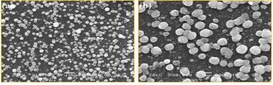
Fig.4. SEM images of CdS thin films deposited at 40 °C(a)10 KX, (b)30 KX
