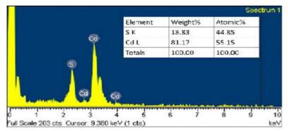
Fig-2: EDS pattern of CdS Thin Film
