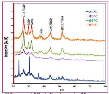
Fig-1: XRD patterns of CdS thin films deposited at different temperatures
