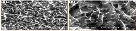
Fig.6. SEM images of CdS thin films deposited at 80 °C(a) 10 KX, (b) 30 KX
