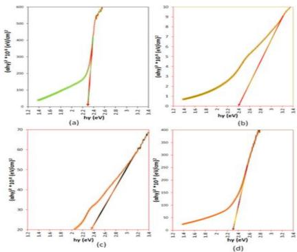
Fig-7: Represents the graphs of band gaps of CdS thin films deposited at (a) 25  $^{\circ}$ C, (b) 45  $^{\circ}$ C, (c) 65  $^{\circ}$ C and (d) 85  $^{\circ}$ C
