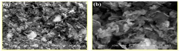
Fig.3. SEM images of CdS thin films deposited at 20 °C(a) 10 KX, (b) 30 KX
