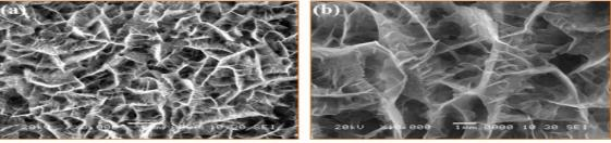
Fig.5. SEM images of CdS thin films deposited at 60 °C(a)10 KX, (b)30 KX
